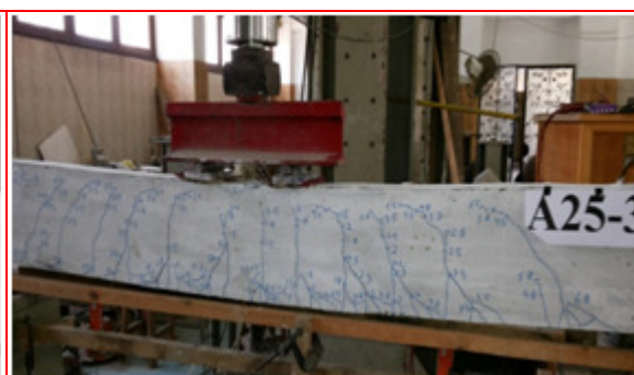
Fig. 4: Crack growth of specimen A25-3
